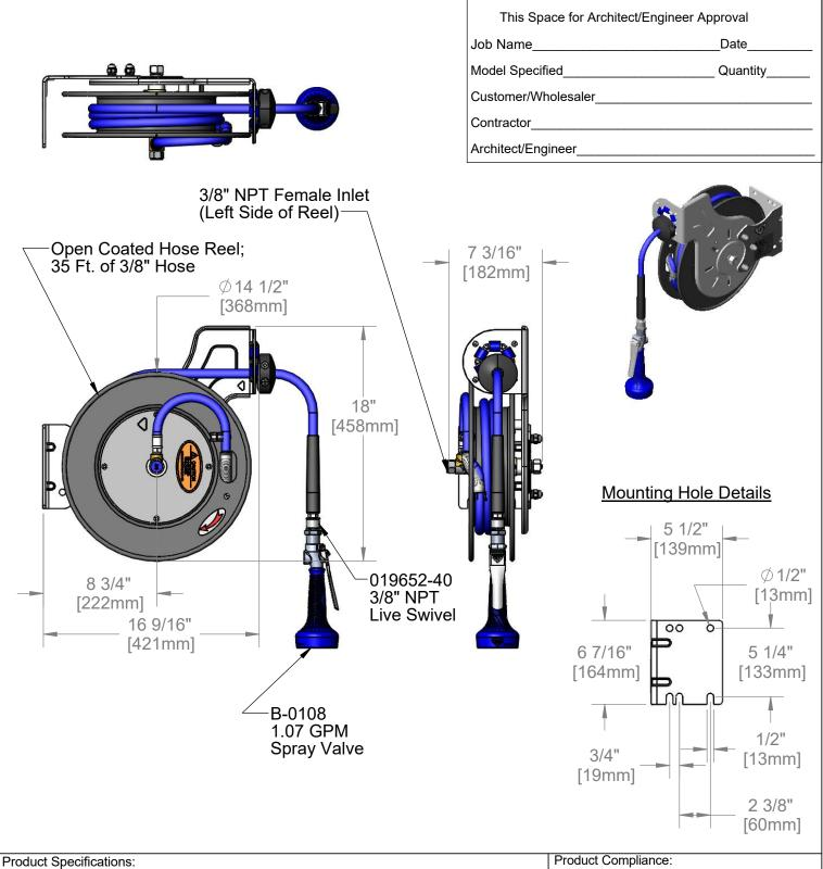
3/8" x 35 Ft. Open Coated Reel w/ 1.07 GPM Spray Valve & Swivel
