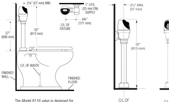
The Model 8116 valve is designed for installations where the water supply is roughed-in 27" (686 mm) above the top of the water closet.
