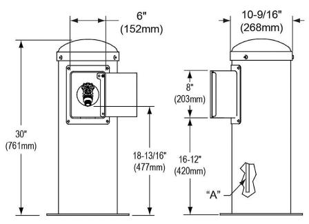
A = 1/2" O.D. UNPLATED COPPER TUBE CONNECT SHUT OFF VALVE BY OTHERS
