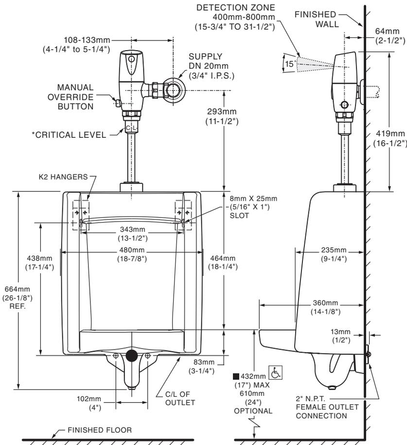
\*Note: The Critical Line (-C-L-) on Vacuum Breaker must typically be a minimum of 6" (152mm) above fixture. Consult Codes for details.
